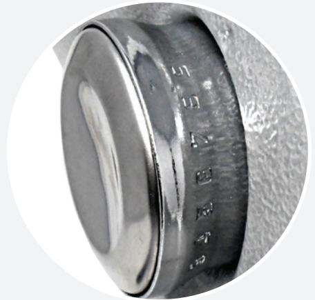
Roller thickness knob with 1 to 9 setting
